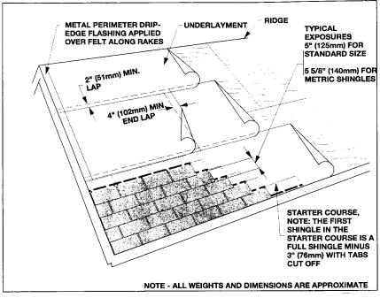
FIGURE 12.7 Three-tab asphalt-shingle roof.
