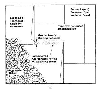
**FIGURE 12.5** Methods of installing single-ply membrane over insulation board: (*a*) ballasted; (*b*) fully adhered; and (*c*) mechanically attached.
