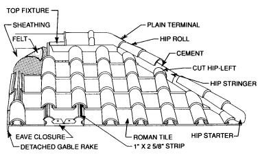
FIGURE 12.10 Roman tile application at hip and ridge of a roof.
