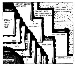
**FIGURE 12.1** Built-up roofing over two layers of preformed insulation board. Three plies of asphalt-impregnated glass-fiber felt, embedded in a continuous application of hot asphalt, overlay a base sheet adhered with asphalt to the insulation. Aggregate surfacing, about  $\frac{3}{4}$  in in diameter, is spread in the top flood coat of asphalt. (*NRCA Roofing and Waterproofing Manual.*)
