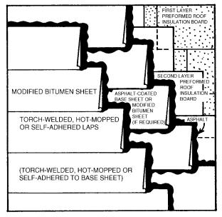
FIGURE 12.3 Modified bitumen roof with a base sheet overlaying two layers of preformed insulation board. (*NRCA Roofing and Waterproofing Manual.*)
